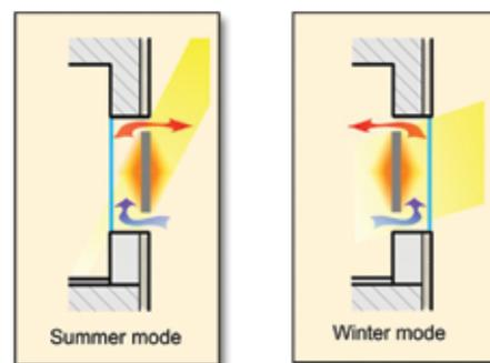
Figure 2. The two modes of operation of the Seasons Window: a) summer (solar protection) mode, left; b) winter (heating) mode, right (Erell et al, 2004).
