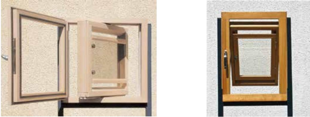
Figure 3. Two experimental prototypes of the reversible window constructed as part of the SOLVENT project (Erell et al, 2004). Photo by: Wolfgang Motzafi-Haller
